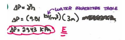
7. The pressure in pipe A shown below is most nearly:
